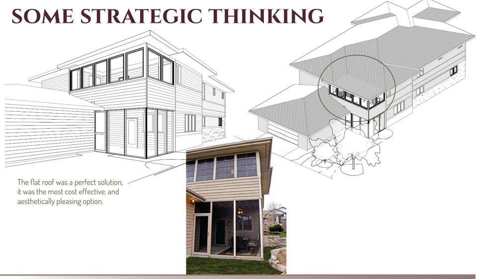
One design challenge that we had to overcome was the roofline. After exploring sloped roof and hip roof options we chose to install a flat roof. The angle of view that most people observe the space from in the alley does not reveal the difference between the flat roof and hip roof of the house to a noticeable extent. It looks good and integrates well into the design, as the eave line was continued to achieve this illusion.
